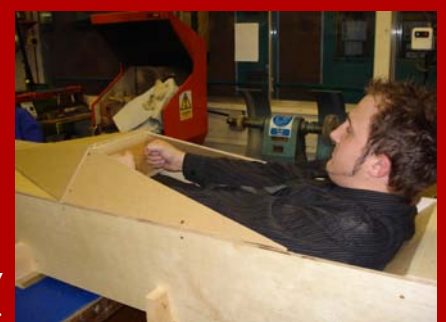
Mr. Hodge tries our ply mock chassis for size.
